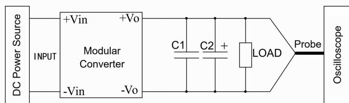
1. The Ripple & Noise test needs the cables in parallel, an oscilloscope that should be set at the Sample Mode, bandwidth 20MHz. 100M bandwidth probe with cap & ground removed. One polypropylene capacitor C1(0.1uF) and one high frequency low impedance electrolytic capacitor C2(10uF) are connected in parallel with the probe.
